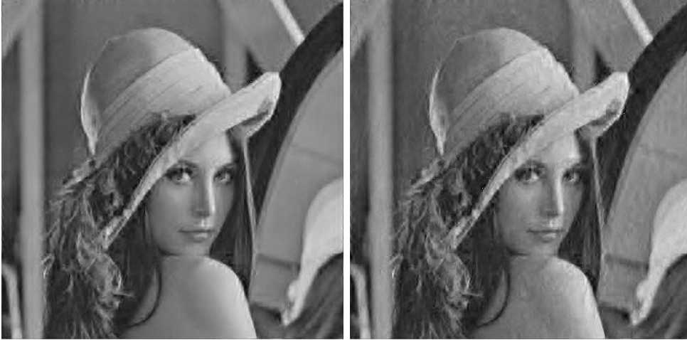
Figure 12. Generalized IFSW approximations with (k_1^*, k_2^*) = (4, 5) : Two parents mapped onto a single child block. Full search for one parent. Search for other parent restricted to quadtrees which lie within a neighbourhood of two quadtrees from the parent block containing the child. (a) No quantization, PSNR = 27.99. (b) (n_1, n_2) = (10, 4) quantization, PSNR = 26.87, R = 45.1 .
