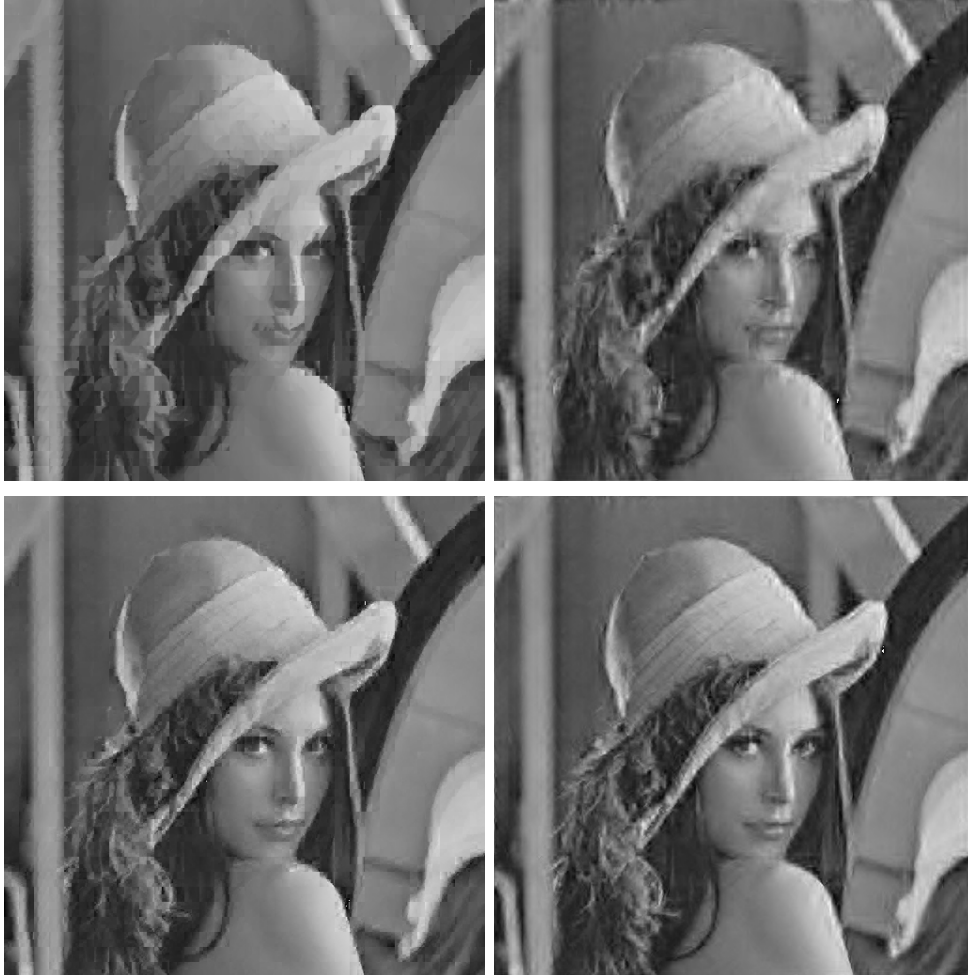
Figure 9. IFSW approximations with (k_1^*, k_2^*) = (4, 5) . Top: “Standard” fractal-wavelet in which \alpha_{ij}^h = \alpha_{ij}^v = \alpha_{ij}^d , same parents. Left: Haar basis (usual IFSM), d_2 = 13.5 , PSNR= 25.6. Right: Coifman-6 basis, d_2 = 13.0 , PSNR= 25.8. Bottom: Three child blocks A_{k_2^*, ij}^\lambda have independent scaling factors \alpha_{ij}^\lambda and parents. Left: Haar basis, d_2 = 11.4 , PSNR= 27.0. Right: Coifman-6 basis, d_2 = 10.7 , PSNR= 27.6.
