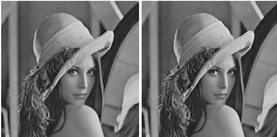
Figure 8. “Standard” fractal-wavelet approximations to the 512 \times 512 pixel Lena image with (k_1^*, k_2^*) = (5, 6) , in which \alpha_{ij}^h = \alpha_{ij}^v = \alpha_{ij}^d , same parents. Left: Haar basis (corresponds to usual IFSM with 16 \times 16 parent blocks \rightarrow 8 \times 8 child blocks); d_2 = 8.2 , PSNR= 29.8. Right: (periodized) Coifman-6 basis; d_2 = 7.9 , PSNR= 30.2.
