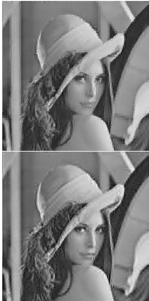
Figure 4.4: Approximations to target image “Lena” using discrete wavelet fractal transform method of Section 5. Domain blocks are 16 \times 16 pixel arrays, range blocks are 8 \times 8 pixel arrays. (a) Haar wavelet basis. (b) “Coifman 12” wavelet basis. (Courtesy of A. Van de Walle.)
