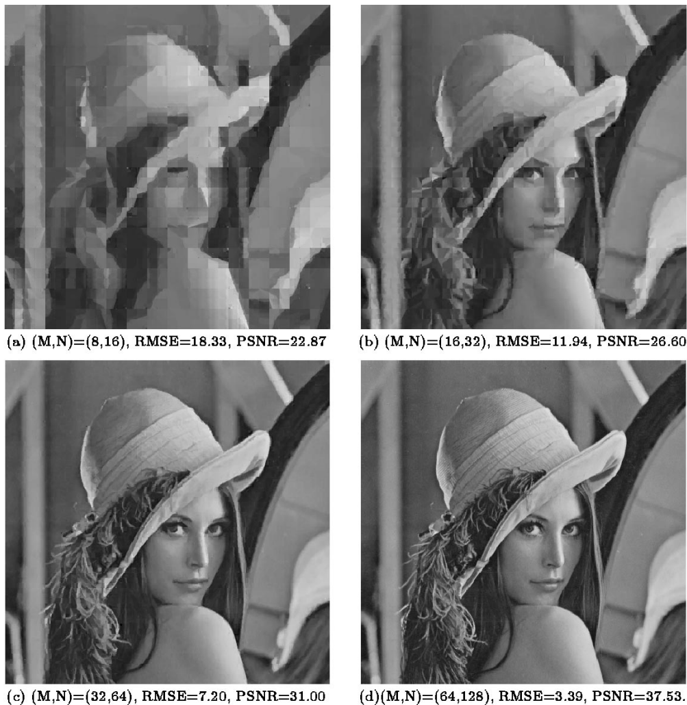
Fig. 3. Fractal representations of the test image of “Lena” for various resolutions values (M, N) . Note that the (64, 128) fractal representation is visually identical to the original image.
