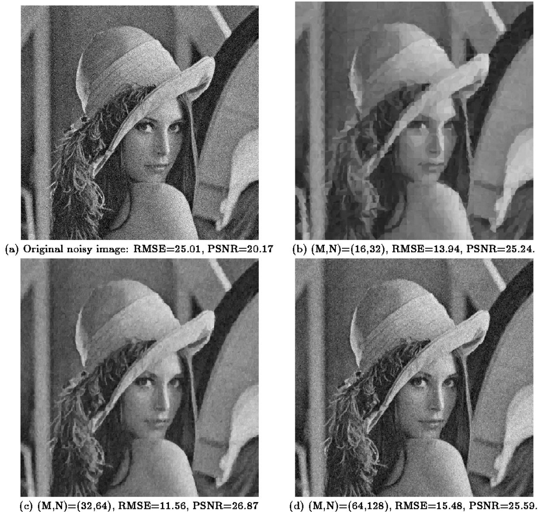
Fig. 4. (a) Original noisy image with noise standard deviation \sigma = 25 and (b)-(d) the standard fractal representations of the noisy image of “Lena” for various resolutions (M, N) .
