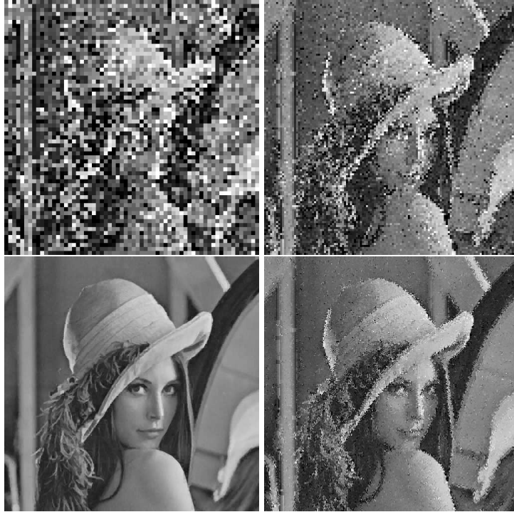
Fig. 3. Starting at upper left and moving clockwise: The iterates u_1 , u_2 and u_3 along with the fixed point \bar{u} of the fractal transform operator T designed to approximate the standard 512 \times 512 (8 bpp) “Lena” image. The “seed” image was u_0(x) = 255 (plain white). The fractal transform T was obtained by “collage coding” using 4096 8 \times 8 nonoverlapping pixel range blocks. The domain pool consisted of the set of 1024 nonoverlapping 16 \times 16 pixel blocks.
