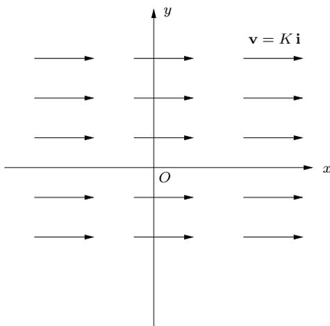
Vector field representing uniform fluid flow in the plane – all fluid particles are travelling at constant velocity
